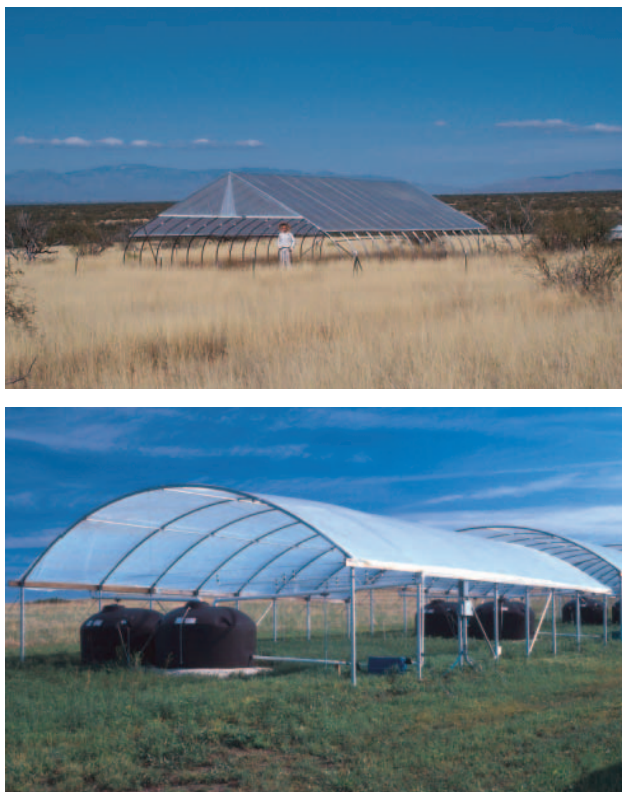
Figure 4. Techniques for experimental manipulation of precipitation. Top: A precipitation shelter in mesquite ( Prosopis ) grassland south of Tucson, Arizona. Twelve experimental plots (1.5 meters [m] by 1.8 m) under each of a total of six such shelters (spread across two soil types) are hand-watered 42 times each year to mimic shifts in seasonal precipitation regimes. Photograph: Nathan English. Bottom: One of 12 precipitation shelters in tall-grass prairie at the Konza Prairie Research Natural Area in northeastern Kansas. Experimental plots (7.6 m by 7.6 m) under each shelter are watered to simulate shifts in seasonal timing of precipitation and changes in the frequency of rainfall events within the growing season. Photograph: Philip A. Fay.
