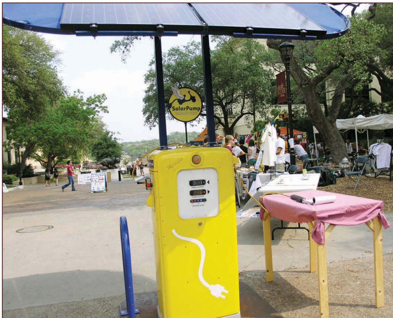
A solar charging station, which charges laptops, cellphones and electric bicycles with a carbon-free energy source, is displayed between the Mitte and Supple buildings in the fall.
