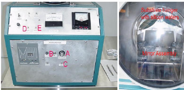
23. Bring the system to air and open the chamber door.
