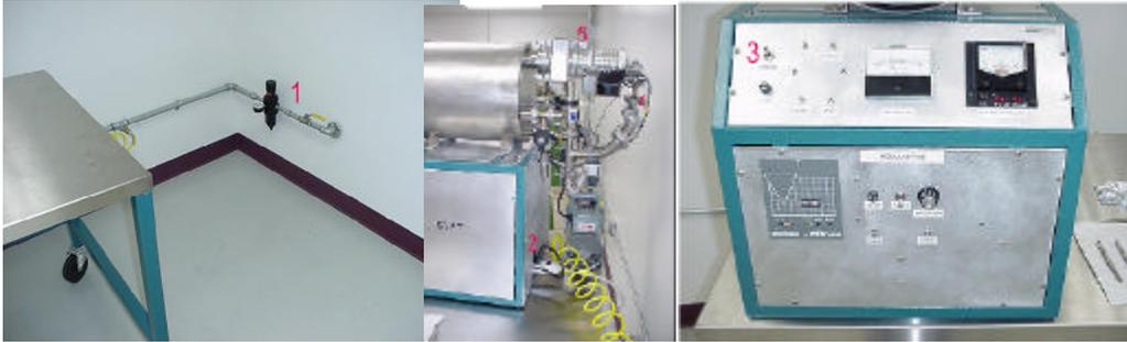
43. Make sure the air pressure valve is open: the air pressure should be 60 psi (1).
