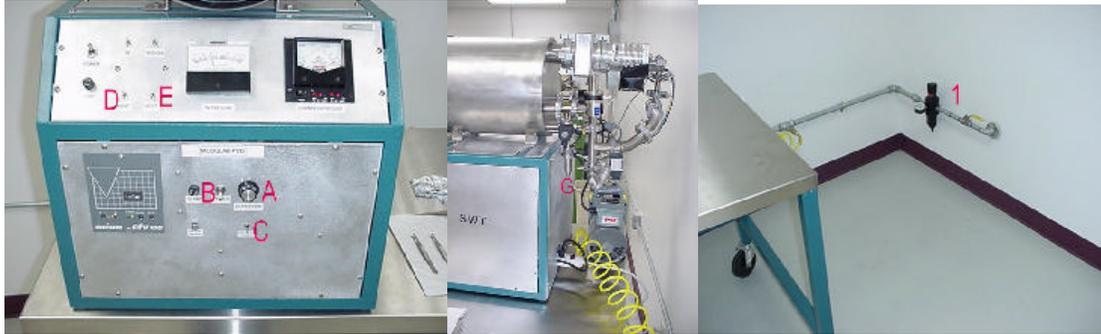
16. Adjust **Power Control CCW** (A) and turn off **Deposition Power** (B).
