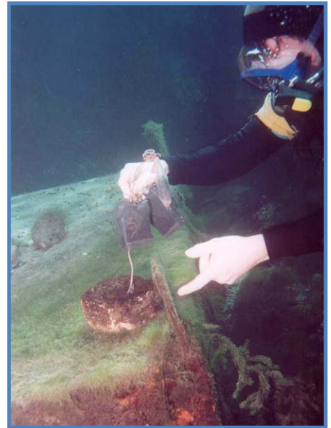
Figure 6: BSEACD staff Hydrogeologist Brian Hunt changes charcoal packets (receptors) at San Marcos Springs. San Marcos Springs are a collection of springs beneath Spring Lake, with depths up to 25 feet requiring scuba equipment to retrieve samples. Photograph taken by Brian Smith.
