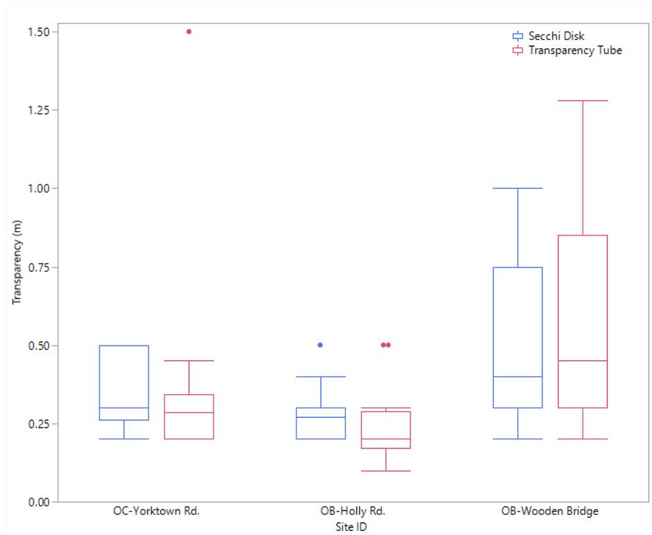
Figure 9. Secchi disk and transparency tube (m) in Oso Creek/Bay watershed (August 2018 to May 2020).
