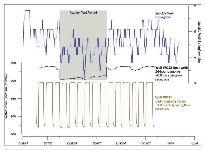
**Figure 12.** Hydrograph of the WC23 pump test with the test period shaded. Both wells WC21 and WC23 show an influence on the flows at Jacob's Well. Location of wells shown on Figure 13. (cfs = cubic feet per second, ft-amsl = feet above mean sea level)
