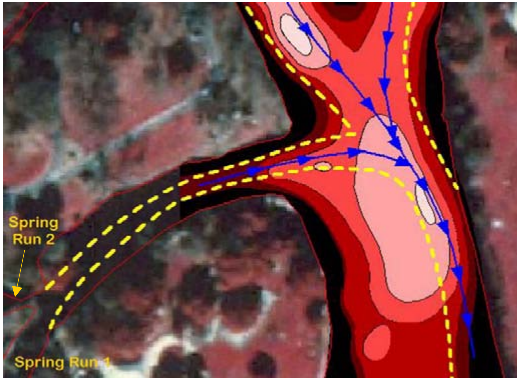
Figure C-12. Close-up of confluence of Spring Runs 1 and 2 in the design to redirect flow in Landa Lake. This is the primary recommendation and would minimize residence time in low quality habitat and reduce water heating during critical low-flows.
