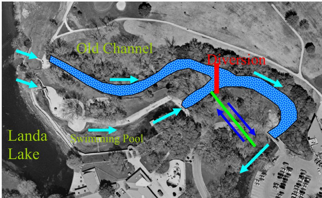
**Figure 6.1** – Conceptual design of an Intensive Management Area on the Old Channel, Comal River
