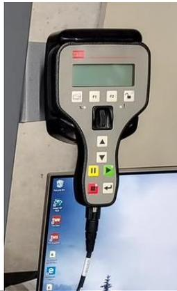
2. Crosshead controls through software can be done one click at a time, or by holding down the clicker for faster movement.
