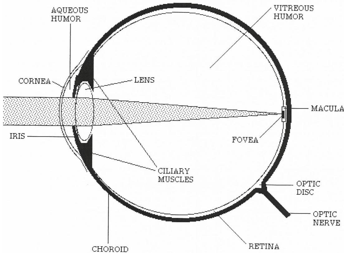
NOTE: The diagram shows a laser beam entering the eye and being focused on the fovea. If the beam power is sufficient, this situation could cause blindness.
