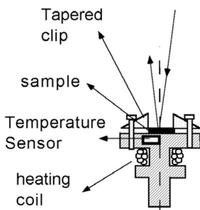
A cernox sensor is mounted in the table just under the sample-platform. Its four contacts are connected to the connector on top of the vacuum window shield by 36 (or 38) phosphor Bronze wires (resistance 65 ohm). As the currents through the sensor are much smaller than those of the heater, thinner wires are sufficient. All leads need to be twisted pairs in order to avoid inductive coupling with the large magnet.
