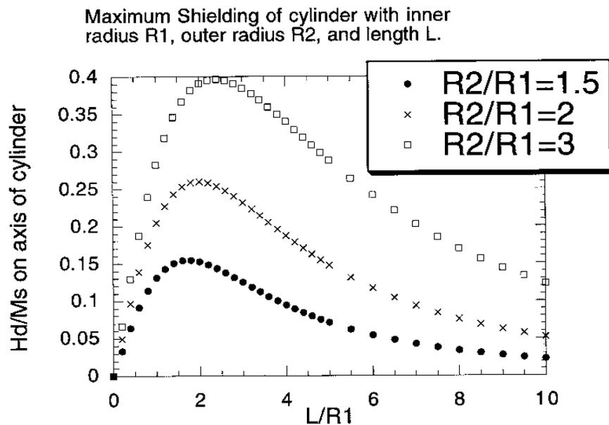
By a more extensive numerical calculations, it can be shown that the field in the wall of the cylinder is almost equal to the field on the axis (at least for  $z=L/2$ ). The magnetic field in the material should be close to zero, as long as the shield does not saturate. This explains roughly the working of the cylinder shield.
