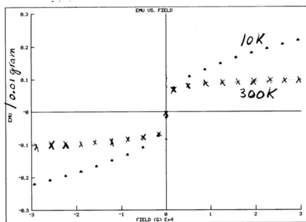
304-Stainless steel is slightly paramagnetic at room temperature. At low temperature its magnetic moment largely increases. Bozorth mentions that the attractive force can be detected by hand in the strong field-gradients of a large electromagnet [20]. The scarce data available of the permeability at low temperature, suggests that 316-stainless steel would be a better choice for the low temperature range.
