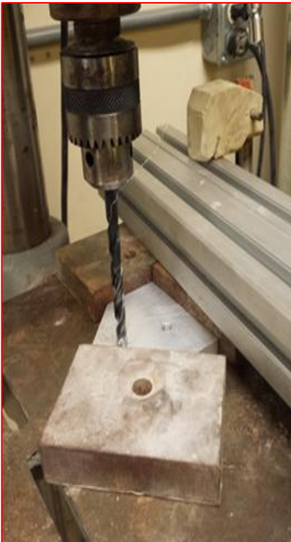
Drill press to create holes in the gusset plates
