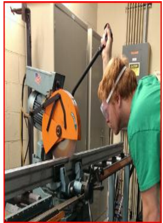
Wet saw to cut extruded t-slots into desired length
