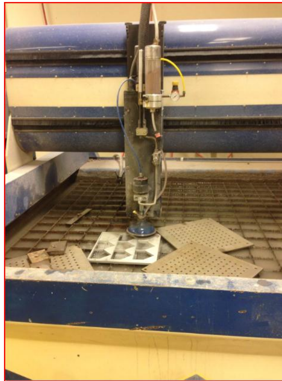
Water jet to cut gusset plates
