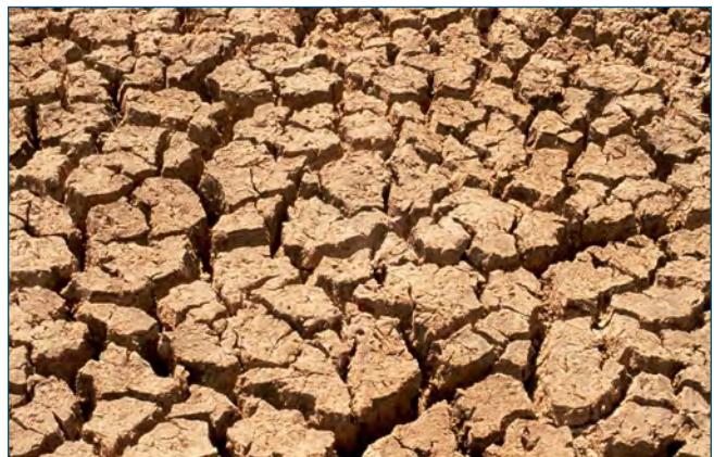
This image demonstrates the shrinking-capacity of clay. Image from CSIRO Science Image .
