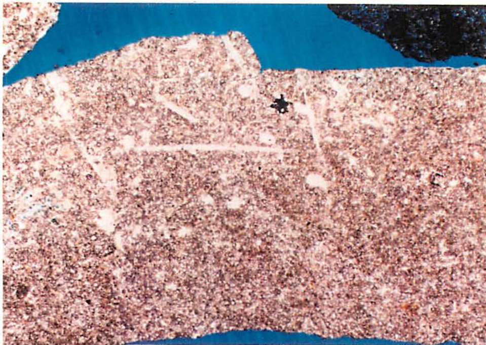
Figure No. 6-2. NBC-1, 561.7-71.7 The rock is a dolomitic chert with no visible porosity. The rock is from the Person Formation above the Regional Dense Member. 20x
