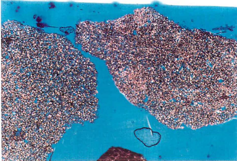
Figure No. 6-30. NBB-1, 706.7-11.4 Type 3 dolomite with intercrystalline, moldic, and vuggy porosity. Porosity is high but the pore diameters are small. 40x
