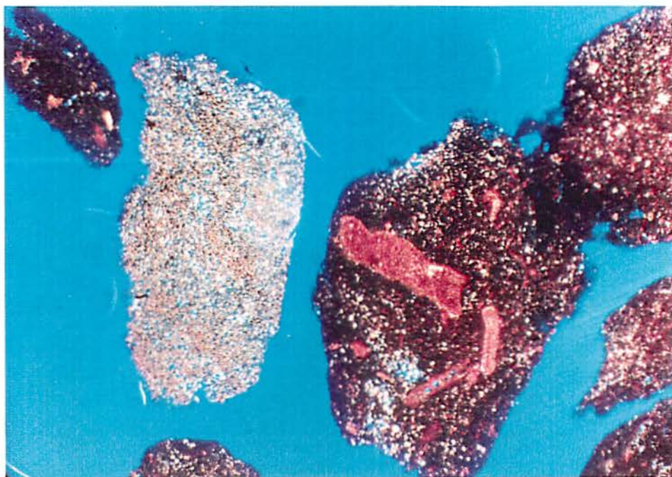
Figure No. 6-7. NBA-1, 586-96 The very fine dolomite on the left side of the photomicrograph has medium porosity. Pore types are intercrystalline and vuggy. However, the pore diameters are so small that the permeability is very low. The rest of the cuttings are Type 1 and 2 limestones. The rock is from the Person Formation above the Regional Dense Member. 20x
