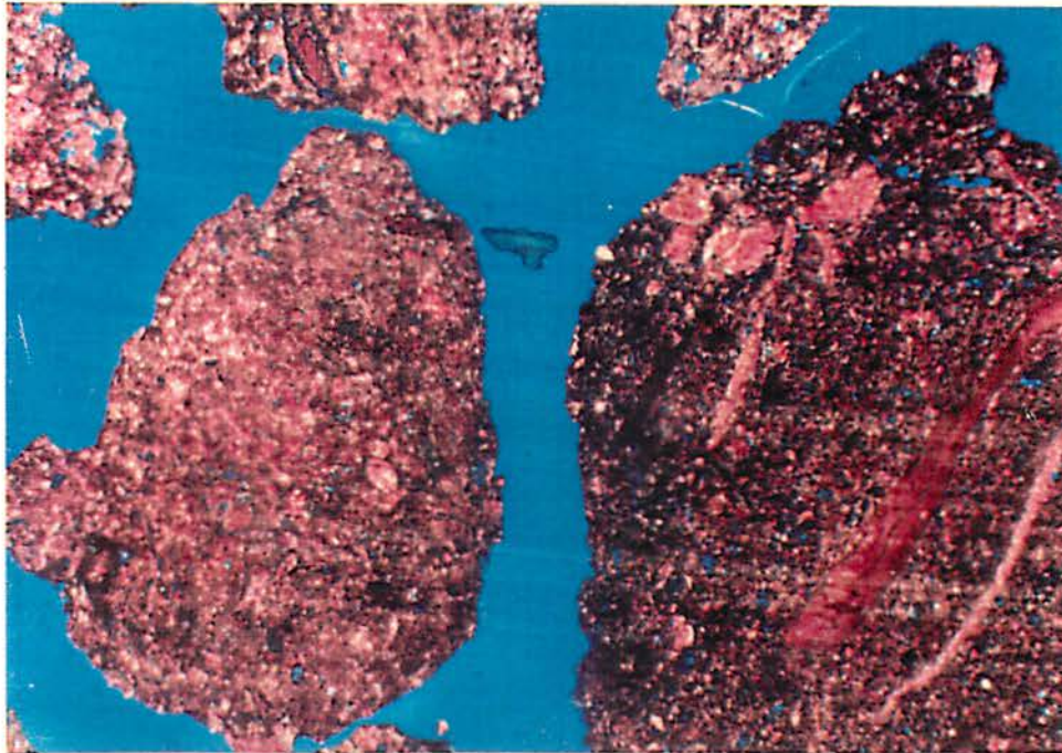
Figure No. 6-3. NBC-1, 540.7-51.7 The limestone is a shaly, fossiliferous packstone. Isolated, moldic porosity is scattered throughout the cuttings. Permeability is very low. The rock is from the very top of the Person Formation. 20x
