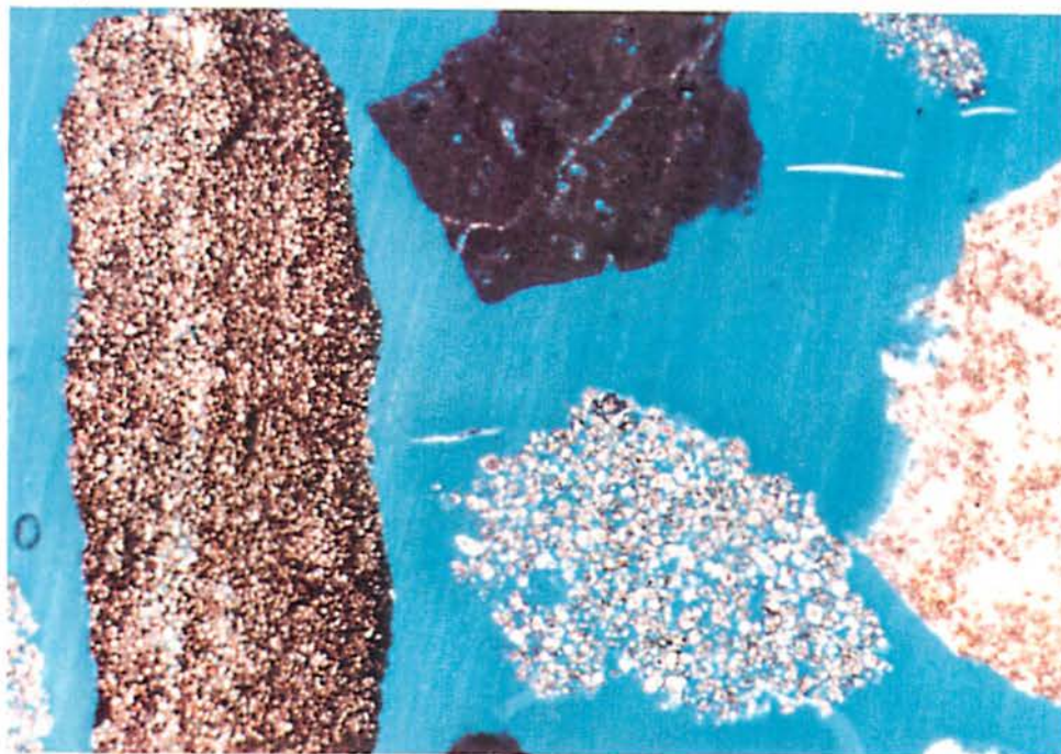
Figure No. 6-22. NBA-1, 516.2-26.2 A shaly, Type 2, very fine dolomite is on the far left. Type 4 dolomite (middle bottom), Type 2 peloidal, packstone dolomite (top right), and dolomitic chert (right) are also pictured. 40x
