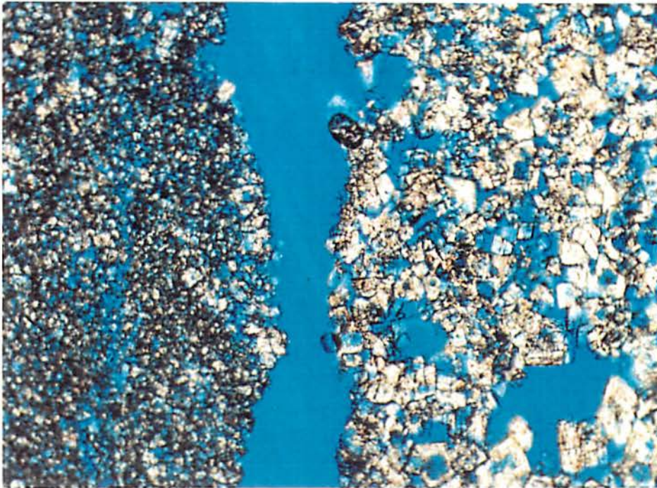
Figure No. 6-11. SMD, 668-79.5 The very fine dolomite on the left side has abundant intercrystalline porosity. The very fine to fine dolomite cutting on the right has abundant moldic intercrystalline and vuggy porosity. The cuttings are from the Kirschberg Evaporite and Dolomitic Members of the Kainer Formation. 100x
